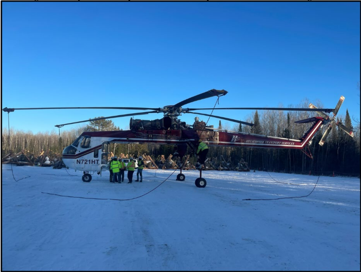
Fig. 13. Heavy-Lift Helicopter Used for Transport and Placement of Log Jacks
