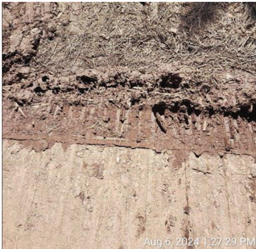
Figure 11. The photo of soil compaction left after the removal of the timber matting along an access route on the Bad River Reservation. The traffic along the matting pushed softer soils out from under the matting (built-up mud towards the top of the picture) and then compressed the soils that remained to the point they were as hard as the timbers that left the pattern on them (bottom of the photo).
