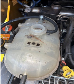
Coolant reservoir with missing cap
