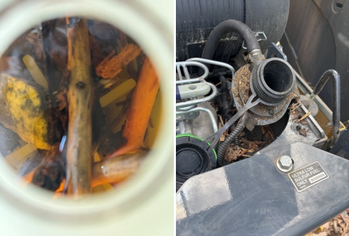
Right Photo: Coolant reservoir filled with sticks and rocks. Left Photo: Remnants of debris around fuel intake
