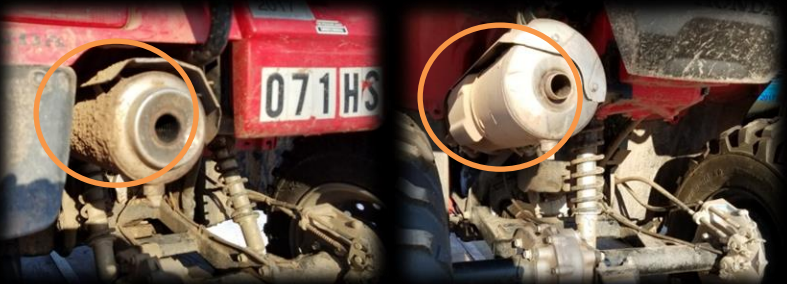
Areas where dirt may be missed when washing include up in wheel wells and around mufflers (left). The ATV on the right has been properly cleaned.
