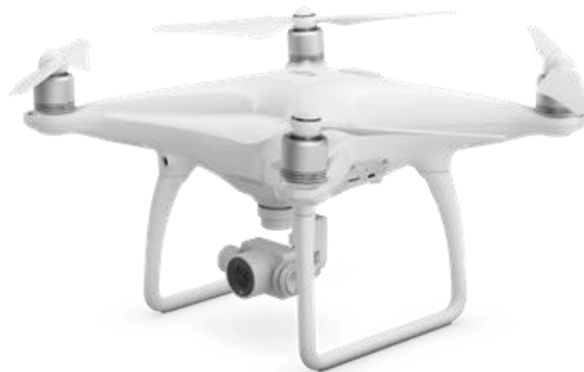
DJI Phantom 4, Bad River Wildlife Precise hovering abilities 28-minute flight time, 3 mile range
