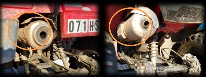
Areas where dirt may be missed when washing include up in wheel wells and around mufflers (left). The ATV on the right has been properly cleaned.
