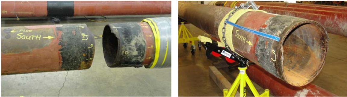
Guillotine rupture of ExxonMobil pipeline, Laurel, Montana, 2011 45
